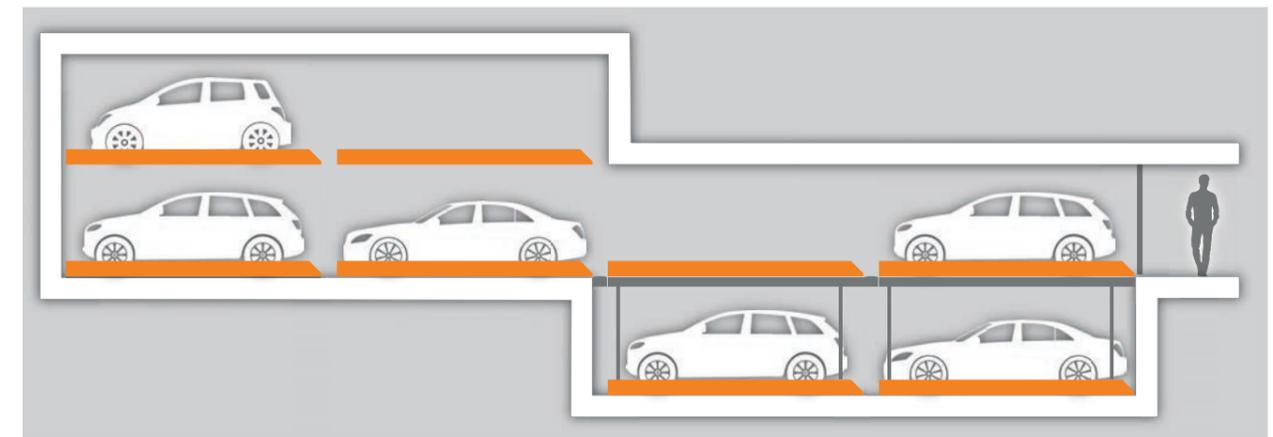
All TrendVario-plus models can be combined any way you like, one after the other, in up to 4 rows. The “plus” stands for the model that can be driven on.
