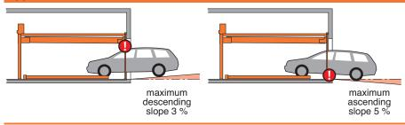
The illustrated maximum approach angles must not be exceeded. Incorrect approach angles will cause serious maneouvring & positioning problems on the parking system for which the local agency of KLAUS Multiparking accepts no responsibility.
