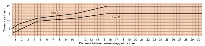
65 Intermediate values are to be taken out the diagram and must be rounded-off to mm.
